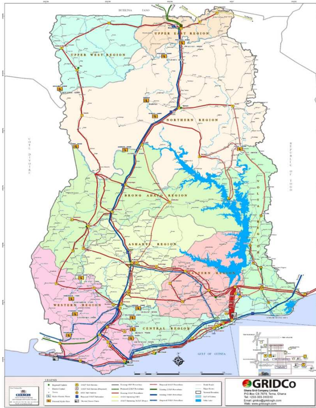
Figure 4: Map of Ghana indicating the locations of major power plants and the interconnected lines for power distribution (Source: Ghana Grid Company, GridCo).
